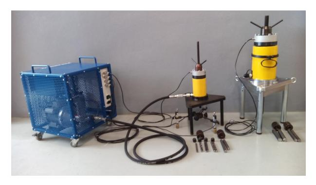
The system consists of driven hydraulic unit HC-17 and two test frames for forces up to 50kN and 135kN. The hydraulic unit also contains a measuring unit with all connections on single panel.
