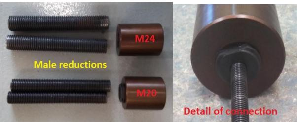
All adapters and reducers are made from hardened steel.
